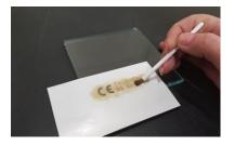
Apply fluid to the stencil with the brush provided, making sure that all the letters and numbers are filled. Leave fluid in place for between 25 and 90 seconds.
