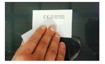
To avoid finger contact with the glass, use the piece of backing material to press the stencil firmly against the surface to ensure a tight bond.
